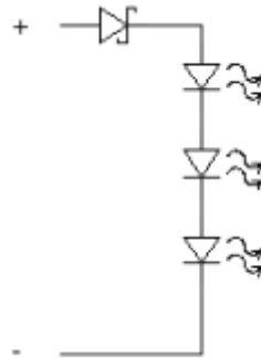
Picture 9. Serial Connected Schotky Diode to LED for Reverse Voltage Protecting
