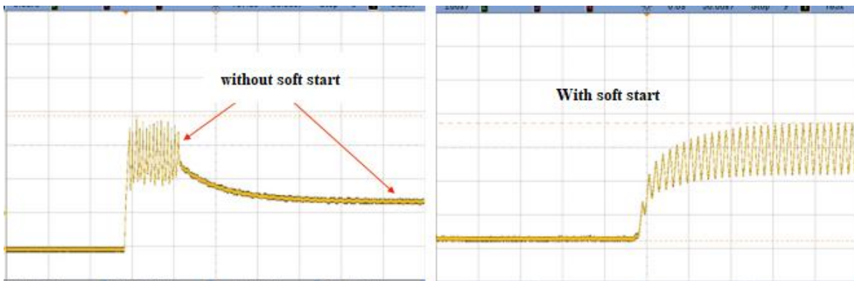
Picture 5. Current Behaviour With Soft Start and Without Soft Start
