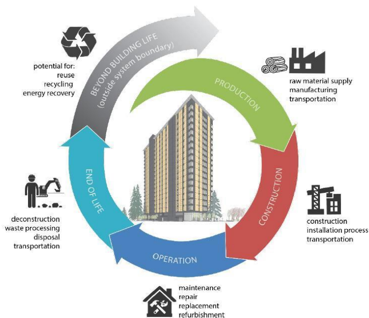
Figure 1. Schematic representation of Building Lifecycle Assessment Phases [6].
